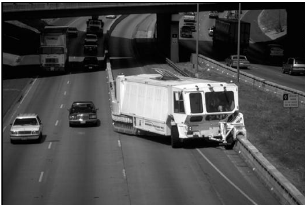
Figure 6-24. Movable Barrier Used in Dallas. (9)
