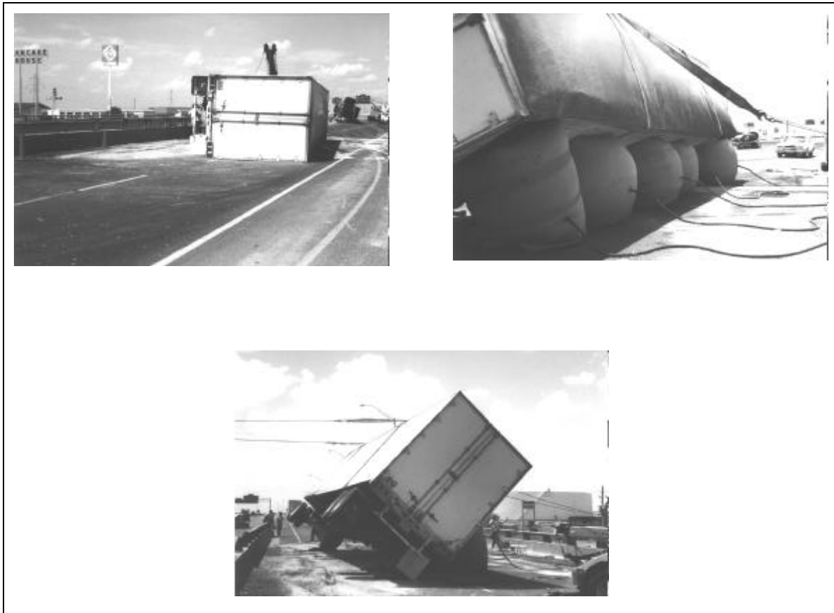
Figure 8-4. Air Bag Use to Overturn Tractor Trailer.
